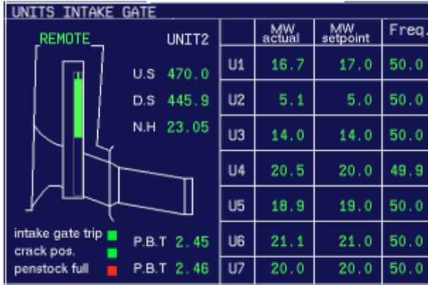
Figure 2: Turbine monitor screen of unit 2 intake gate
