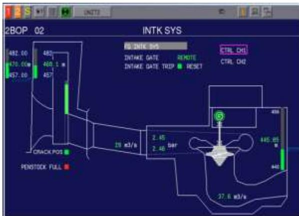
Fig 3: Turbine monitor screen of unit 2 intake system
