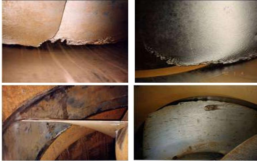
Figure 1: Cavitation areas in machine runner chamber
