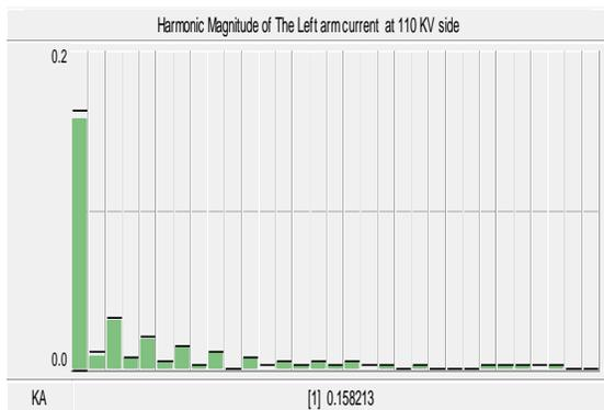
**Fig. 5. Harmonics of the total current at 110 KV side.**
