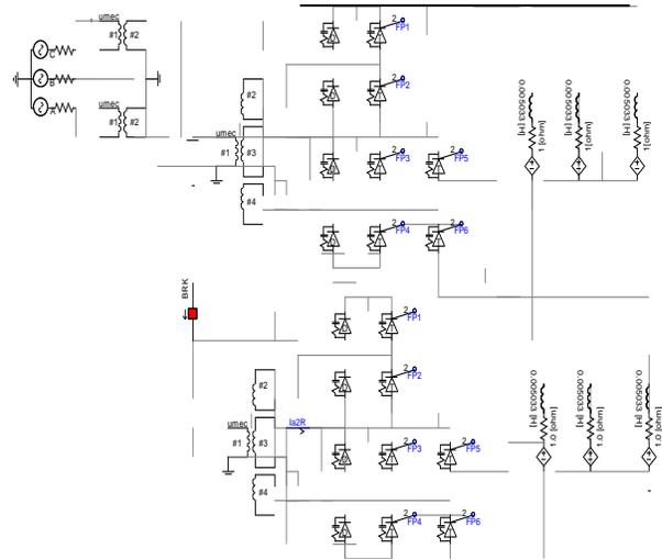
Fig. 2. The PSCAD model of electric railway system connected to V/V transformer.
