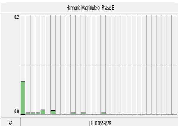
Fig. 10. The current harmonics of phase B on 110 KV side.
