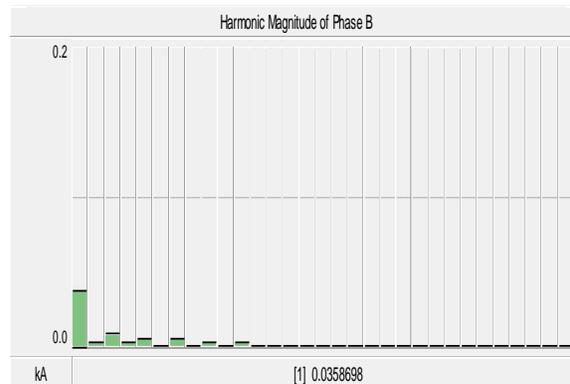
**Figure 7. The current harmonics of phase B on 110 KV side.**
