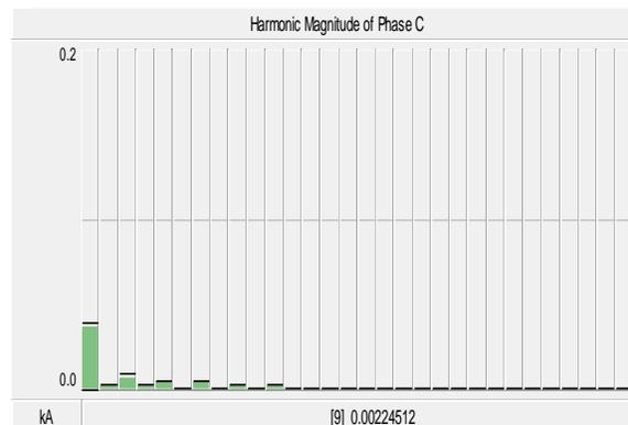
**Figure 8. The current harmonics of phase C on 110 KV side.**
