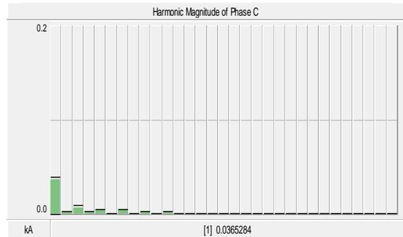
Fig. 11. The current harmonics of phase C on 110 KV side.
