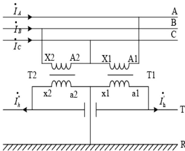
Fig. 1. The wiring diagram of three-phase V/V transformer.
