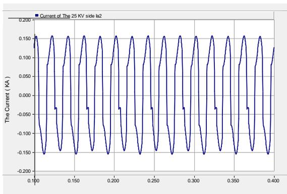
**Fig. 4. Current waveform on 110 kV side of traction substation transformer.**
