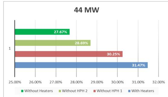
**Figure 7: The overall power plant efficiency for 44 MW.**
