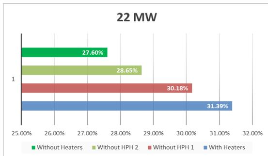
Figure. 11: The overall power plant efficiency for 22 MW.
