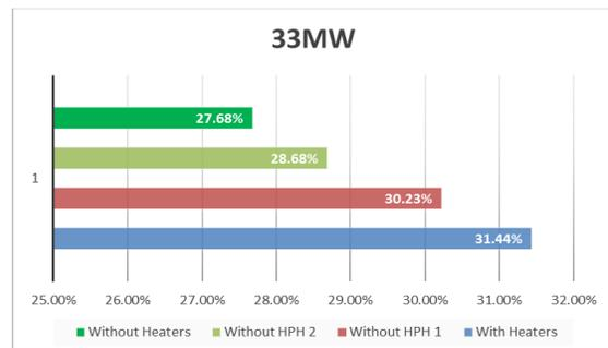
**Figure 9: The overall power plant efficiency for 33 MW.**
