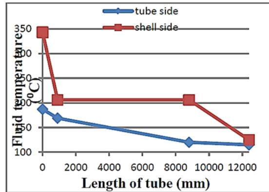
Figure 2: The effect of the tube length to the HP heaters to rise in temperature
