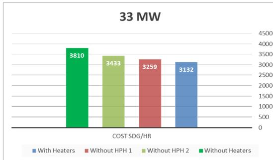
Figure.10: The cost SDG per hour, for 33 MW.
